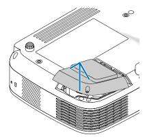
3. Loosen the two screws securing the lamp housing until the phillips screwdriver goes into a freewheeling condition. The two screws are not removable.
